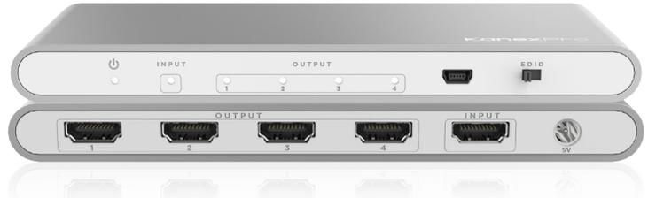
The KanexPro SP-HD20-1X44K is an one input, four output HDMI Distribution Amplifier engineered to split 4K quality videos or high res images from one source to four HD 4K displays with resolutions up to 4K@60Hz and HDCP2.2 specifications. Built-in EDID management allows optimal resolution to be selected and properly outputted to avoid response time and delays.
